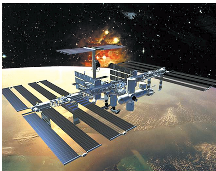
Artist's rendition of the fully assembled International Space Station Alpha . The pressurized volume of the station following a 5-year, 45-mission sequence of assembly will be roughly equivalent to the space inside two Boeing 747 jet airplanes. NASA image.
