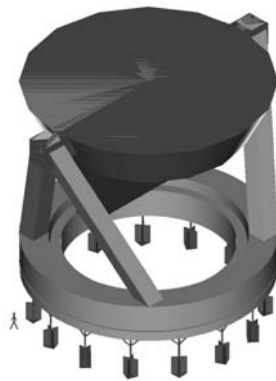
Fig.7 main mirror support structure
