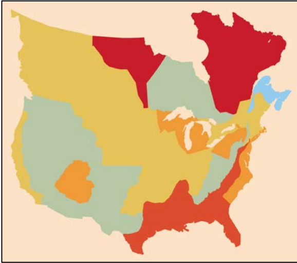
Figure 3: Relative risk from strong electric field fluctuations in the US and Canada based on ground conductivity models. Red and blue represents the highest and lowest risk regions, respectively.
