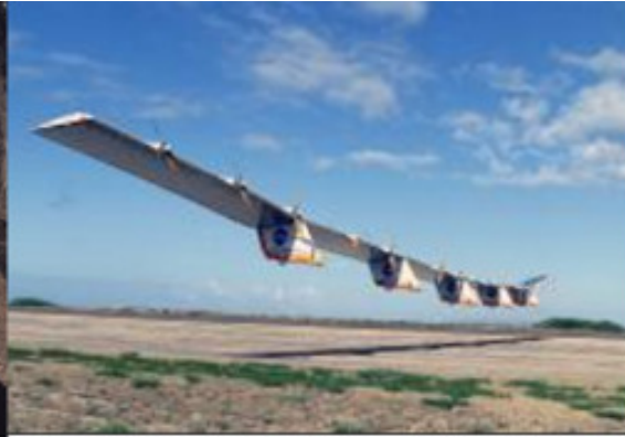
Helios prototype flying wing moments after takeoff to begin its first test flight on solar power—it set a high altitude record of 96,863 ft. in a 2001 flight from the U.S. Navy's Pacific Missile Range Facility on Kauai, HI.
