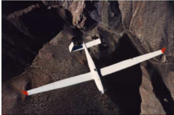
A Burt Rutan Raptor Demonstrator that executed high-altitude, long-endurance UAV flights, satisfying rigorous performance criteria on flights of up to 65,000 ft. and over 48 hours endurance.
