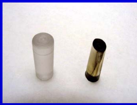
0.74 gm Lexan Projectile slid to rest from 2.06 k/s
